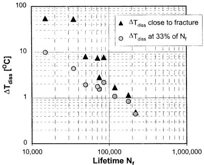
Figure 6: Relation of  $\Delta T_{diss}$  to fatigue life N<sub>f</sub> evaluated at 30 Hz and R=0.06-0.17
