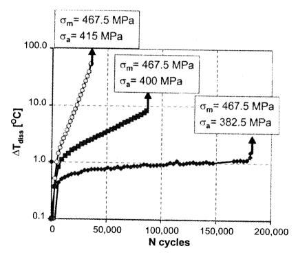
Figure 4:  $\Delta T_{diss}$  (N) curve evaluated in fatigue experiments at low R-ratios for amplitudes  $\sigma_a$ : 382.5 MPa, 400 MPa, 415 MPa (30 Hz,  $\sigma_m$ =467.5 MPa)
