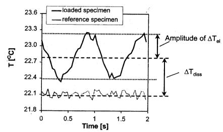
Figure 2: Time dependent oscillation of temperature due to thermo elasticity and evaluation of  $\Delta T_{diss}$
