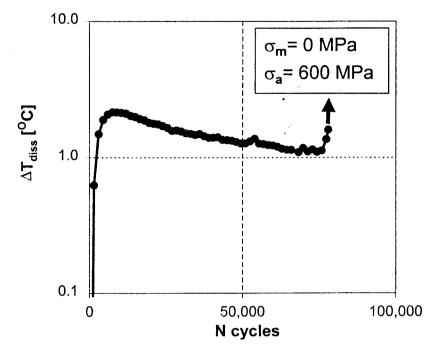
Figure 5:  $\Delta T_{diss}$  (N) curve evaluated in a fatigue experiment at R= -1 ( $\sigma_m$ =0 MPa,  $\sigma_a$ =600 MPa, 30 Hz)
