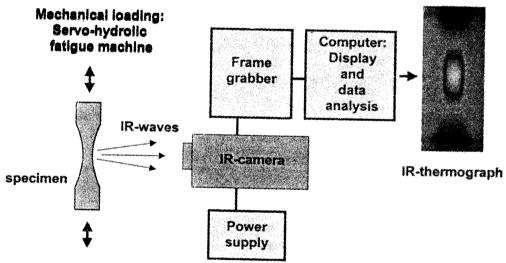
Figure 1: Experimental set-up used for passive thermography
