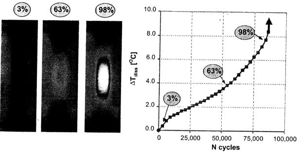
Figure 3:  $\Delta T_{diss}$  (N) curve evaluated in a fatigue experiment ( $\sigma_m$ =467.5 MPa,  $\sigma_a$ =400 MPa, 30 Hz); IR-thermographs measured at 3%, 63%, 98 % of the fatigue life N<sub>f</sub>=85,852 cycles
